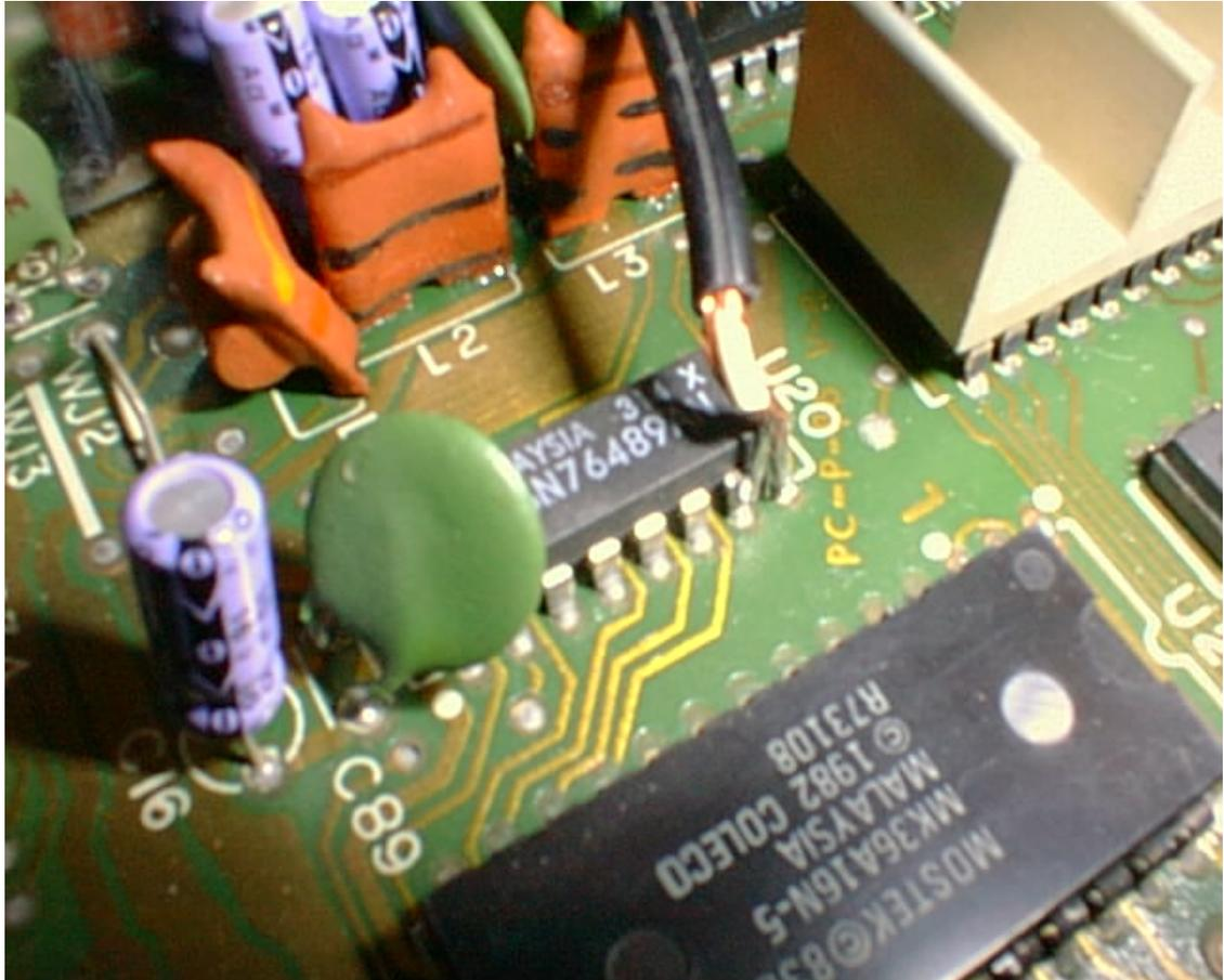
Unfortunately, the actual solder connection is a little blurry in that picture. This one is tricky, and tinning the wire is essential.
